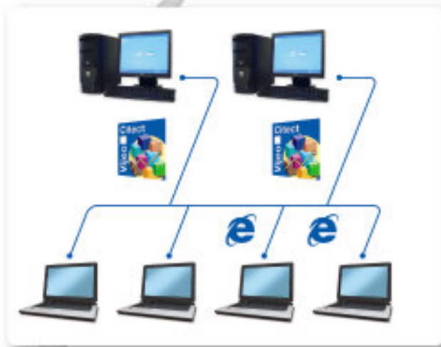
Redundant architecture with 2 servers and 2 Web clients
